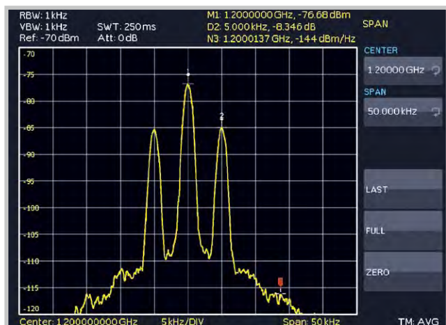
Absolut Marker M1; Delta Marker D2; Noise Marker N3
